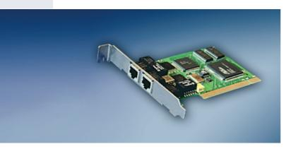
PCI card Tahoe 931 and Tahoe 932 cards are equipped with, respectively, one and two V.35 interfaces. They may work in both unframed or framed mode.
